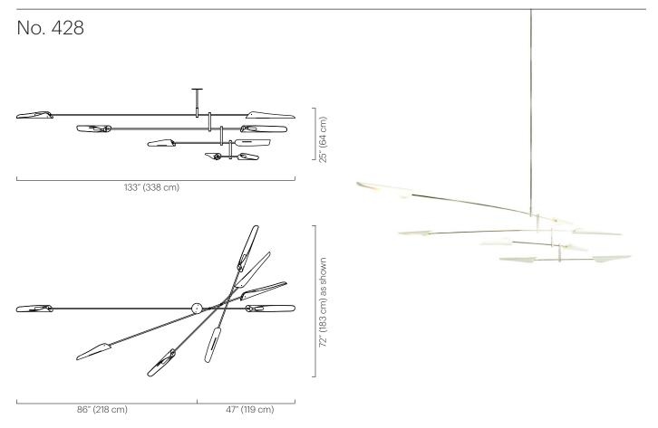
The Sarus Mobile is a carefully balanced fixture, featuring four tiers of differing lengths. Each tier has one large and one small Sarus shade. Tiers scissor open when installed; arrangement is adjustable on site. Shades swivel 320° to cast light directionally.
