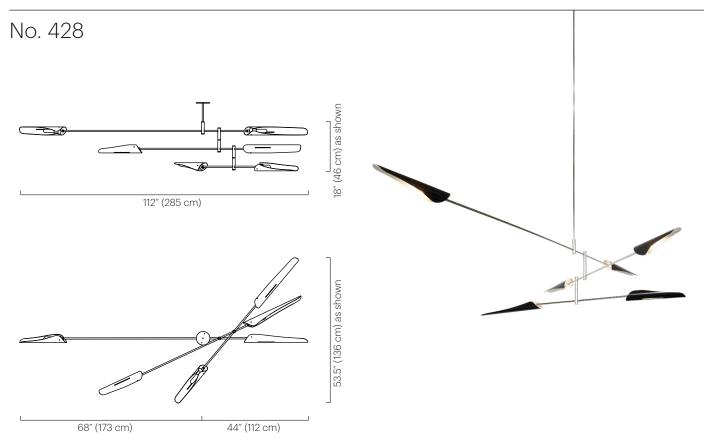
The Sarus Mobile is a carefully balanced fixture, featuring three tiers of differing lengths. Each tier has one large and one small Sarus shade. Tiers scissor open when installed; arrangement is adjustable on site. Shades swivel 320° to cast light directionally.
