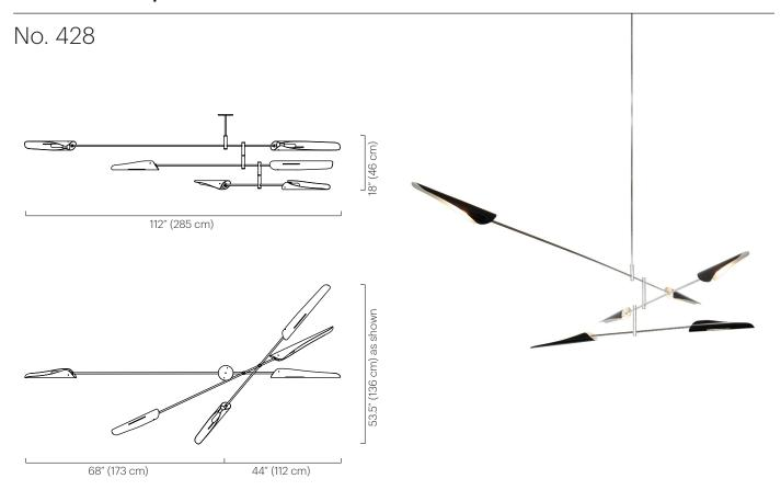
The Sarus Mobile is a carefully balanced fixture, featuring three tiers of differing lengths. Each tier has one large and one small Sarus shade. Tiers scissor open when installed; arrangement is adjustable on site. Shades swivel 320° to cast light directionally.
