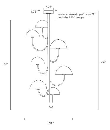
Timeless modern hand-blown glass is suspended vertically in space providing distinct dimmable illumination. The light is illuminated by 7 120V AC direct drive LED modules with no external driver needed. It can be wired to a dimmer switch, providing smooth full range dimming and is compatible with most Triac and ELV dimmers. The light is UL certified.
