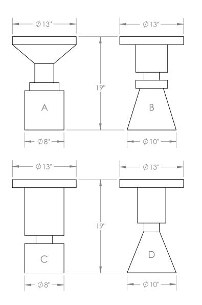
Like chess pieces dotted across a board, these sculptures can be placed throughout a room. Used as side tables or stools, they are made to work in series or alone. Metal stools are made from cold rolled steel, brass plated and finished with a hand rubbed patina. Wood and parchment stools are hand-turned, finished and sealed with waterresistant lacquer.
